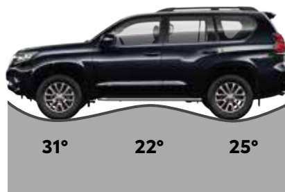
Approach, ramp break-over and departure angles
